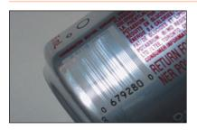
Using uncovered metal surfaces as a background or for the bars of a symbol. The specular reflectance of the substrate can cause problems, and a solid background should be printed to provide contrast and eliminate this problem.
