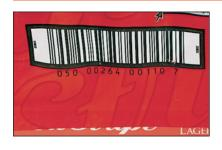
Printing barcodes onto film which is distorted as it is used as shrink wrap.
