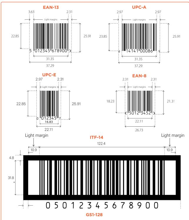
The overall dimensions of a GS1-128 barcode will vary according to how much data is encoded, but when printed at 100% the module width of a GS1-128 symbol is 1mm and bar height is 32mm\*. See method of calculating length on Appendix 6, page 48.
