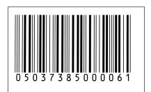
Incorrect adjustment for ink spread (the bar width reduction). The printed bars are out of specification, either being too narrow or too wide.
