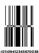
GS1 DataBar Stacked Omnidirectional
