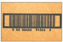
Poor quality substrates are substituted for the original specification, resulting in loss of quality, often greater ink spread, or the appearance of voids in the bars. A darker coloured substrate, for example, could result in insufficient contrast.
