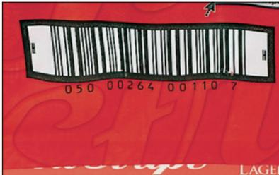
Printing barcodes onto film which is distorted as it is used as shrink wrap.
