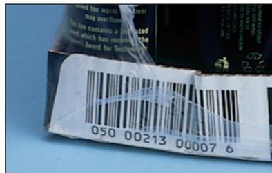
Printing barcode on to packaging or a label which is then distorted.
