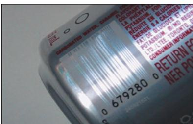
Using uncovered metal surfaces as a background or for the bars of a symbol. The specular reflectance of the substrate can cause problems, and a solid background should be printed to provide contrast and eliminate this problem.
