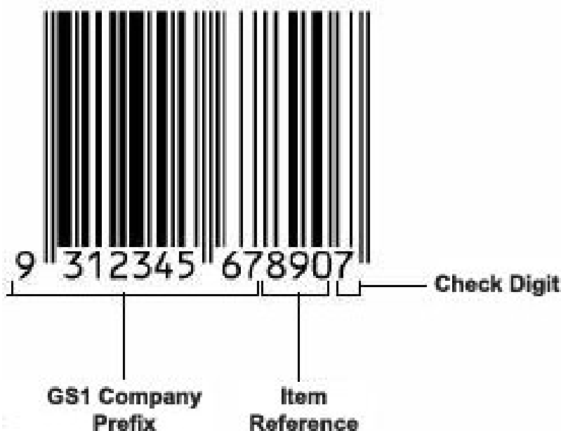
Example of a nominal size EAN-13 Barcode Symbol (diagram is not to scale)
