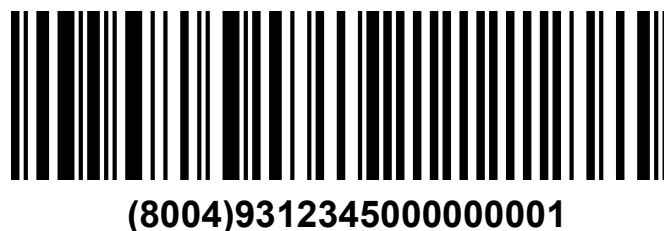
Figure 30: Global Individual Asset Identifier, AI (8004), represented in a GS1-128 Barcode
