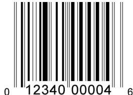
Figure 8: Example of a UPC-A Barcode representing the GTIN-12
