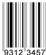
Figure 7: Example of an EAN-8 Barcode representing the GTIN-8
