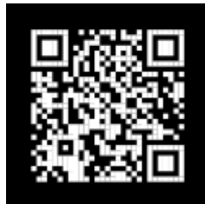
mirror image orientation and reversed reflectance
