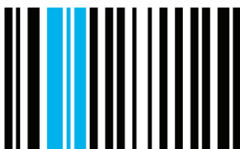
Enlarged section of the first part of a GS1-128 barcode showing the Function 1 character in blue.
